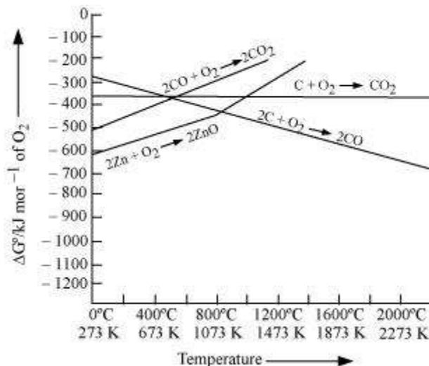
Reduction of ZnO to Zn is usually carried out at 1673 K. From the above figure, it can be observed that above 1073 K, the Gibbs free energy of formation of CO from C and above 1273 K, the Gibbs free energy of formation of  $\text{CO}_2$  from C is lesser than the Gibbs free energy of formation of ZnO. Therefore, C can easily reduce ZnO to Zn.
