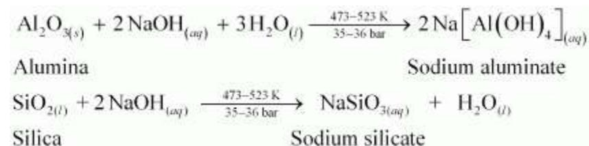
The impurities are then filtered and the solution is neutralized by passing  $\text{CO}_2$  gas. In this process, hydrated  $\text{Al}_2\text{O}_3$  gets precipitated and sodium silicate remains in the solution. Precipitation is induced by seeding the solution with freshly prepared samples of hydrated  $\text{Al}_2\text{O}_3$ .
