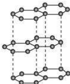
It has  $sp^2$  hybridised carbon, arranged in the form of layers. These layers are held together by weak van der Waals' forces. These layers can slide over each other, making graphite soft and slippery. Therefore, it is used as a lubricant.
