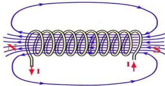
We can determine the magnetic poles formed in a solenoid. The end of the current-carrying solenoid, which attracts North Pole but repels South Pole of a bar magnet, is behaving as south magnetic pole. The other end, which attracts South Pole of a bar magnet but repels the North Pole, is behaving as north magnetic pole. It is because like poles repel but unlike poles attract each other.
